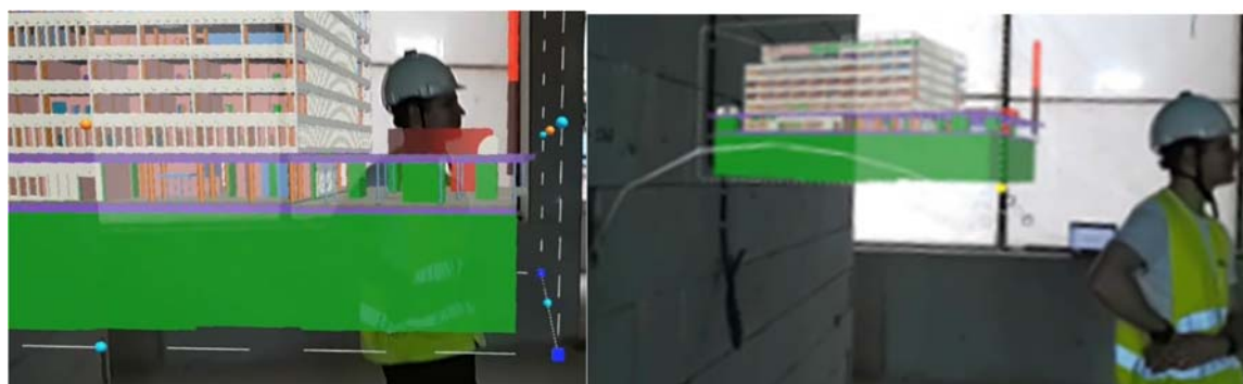
Figure 38. The BIM model is scaled down to optimize the HSO’s visibility and maintain a clear view of the surrounding environment
