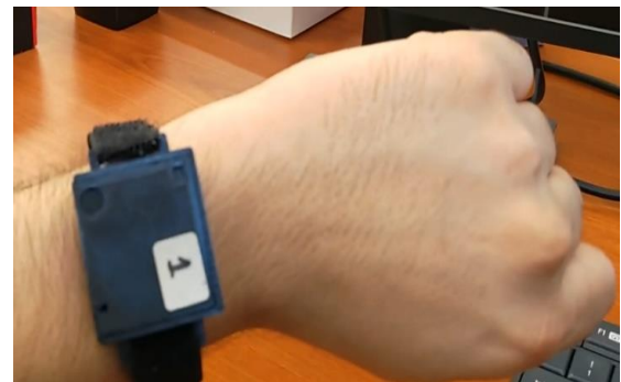
Figure 3b. A special wearable is worn by the site's workers that tracks their location and their heartbeat at all times
