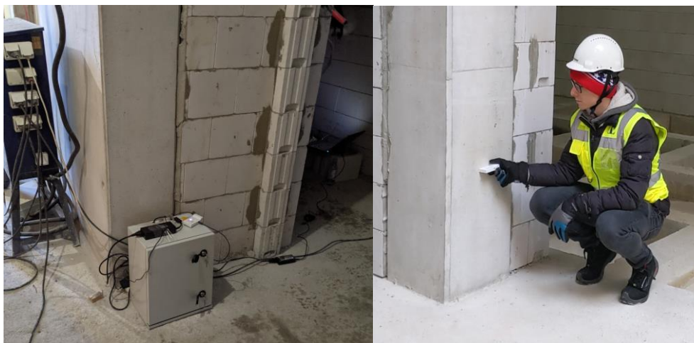
Figure 21. Left: Prototype GWEN in a protective enclosure on the construction site, during the range test. Right: Measuring UWB range on the construction site
