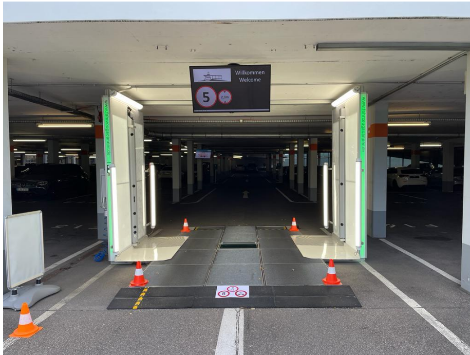
Figure 47. Vehicle scanner as pilot outdoor installation at final user
