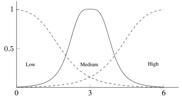
Fig. 3. Membership function for “UV exposure”
