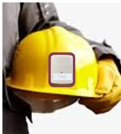
Figure 32. Tag for monitoring the location of hazardous worker situations.
