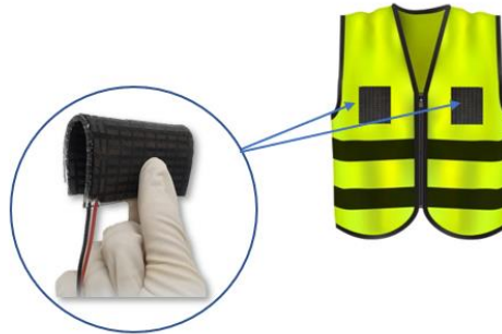
Figure 30. A scheme of high visibility vest with integrated thermoelectric modules
