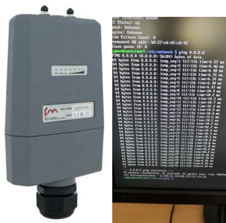
Figure 21. Fluid-mesh transceiver (left), zero IP packets loss when switching between ethernet-WIFI-Ethernet
