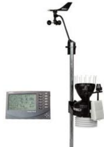
Figure 31. Selected weather station Davis Instruments Vantage Pro2 Plus [source: www.davisinstruments.com ]
