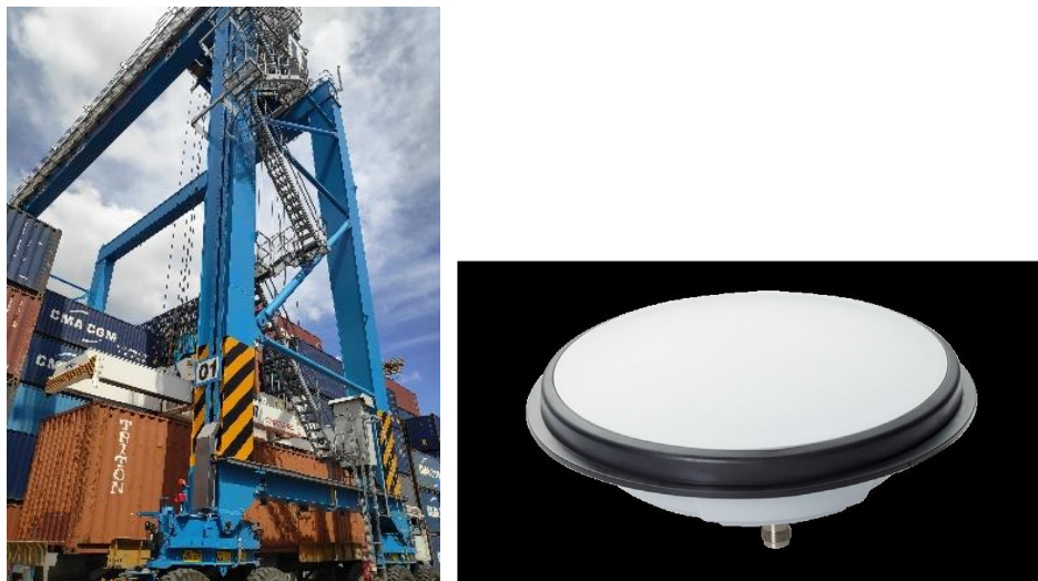
Figure 5. RTG crane (left), and GPS antenna (right)
