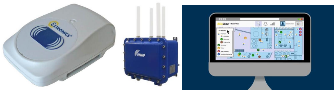
Figure 106. AeroScout suite. Active RFID tags (left), Wi-Fi access points (centre), and MobileView software (right).
