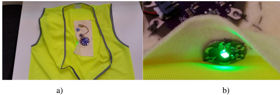
Figure 71. (a) A vest with temperature sensors (b) and LED diode signalling incorrect temperature values [SSW-28].
