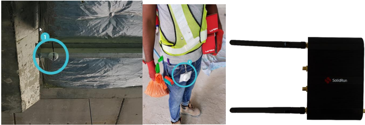
Figure 105. ELA innovation localisation suite. Anchors (left), tags (centre), and gateways (right).
